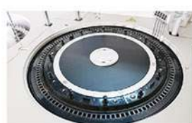
Reaction Tray 37±0.2°C, real-time monitor.
