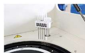
Washing Probe Independent 5-step washing system.
