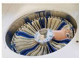
Reagent Tray 2~8°C cooling for 24 hours.
